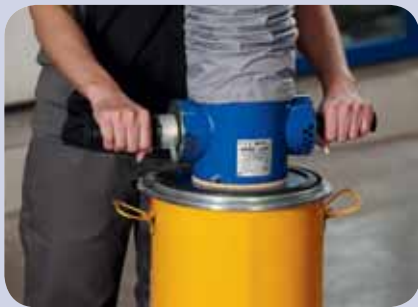
Drum lift, attached to the top of drum
