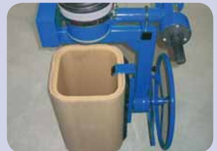
Handling of chimney flue tiles
